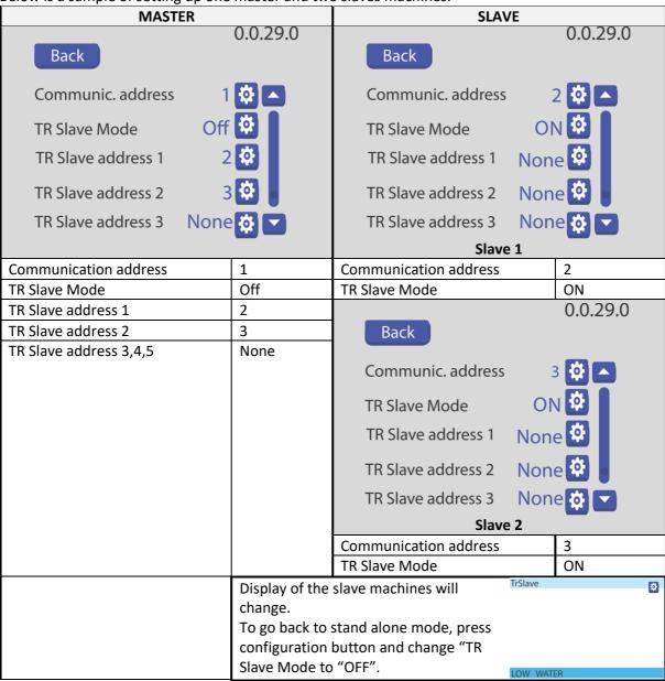
If more then 2 slaves are set, the master machine TR Slave address 3, 4, 5 must be set. The slave machines must be set accordingly to correspond with the master unit.
