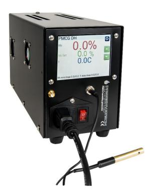
The PMCG generator is a miniature humidity control device for museum showcases and similar small sealed enclosures. This unit can reliably control humidity for individual well sealed enclosures.
