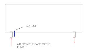
In most applications, locate the sensor near (but not directly in) the air input from the PMCG.
