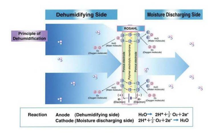
Rosahl has no moving parts. This makes it economical to run, silent and vibration free in operation. Because no liquid water is involved in the process, it is maintenance free making it suitable for us in remote locations or where servicing is expensive. The membrane has a long operating life and has been tested to work from -10 to +50C
