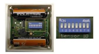
For better orientation, radio humidity transmitters within range transmit their current code to the device. You can recognise this by a short beep and two flashing dots in the display next to the address code. Caution: If several radio humidity transmitters are within range, different codes are displayed.
