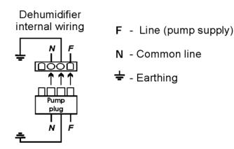
If a condensate pump is used, it must be connected to the socket under the water pan of the dehumidifier. Only then it is possible to turn it back on.
