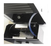
⇒ Now insert the pump plug into the corresponding socket on the rear wall of the unit behind the tank. Insert the water tank as usual;
