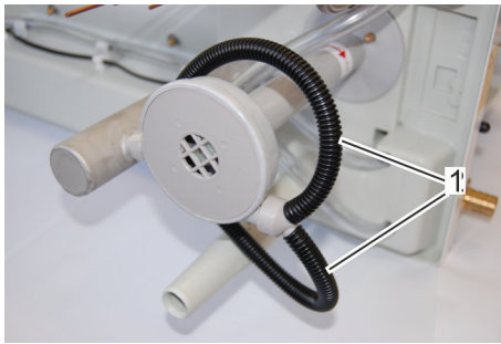
Fig. 50: Attaching the pump hoses
