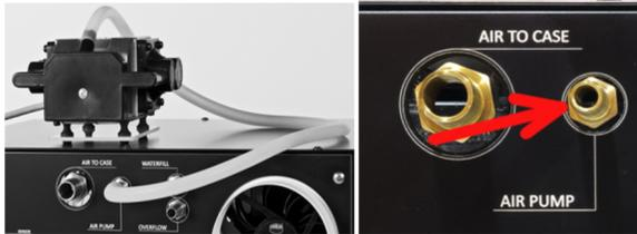
The air pump is supplied with 78"/2m long silicone hose. **The length of this hose should not be adjusted, otherwise the machine may not work properly**, especially with a low humidity setting. The other end of the hose should be connected to the machine fitting labeled "AIR PUMP".
