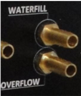
Turn the unit on. Attach the hose with funnel to the WATER FILL port and slowly add water.
