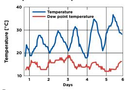
Dew point temperature is kept below surface temperature, preventing condensation and moisture damage.
