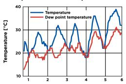
Condensation occurs when surface temperature and dew point temperature are equal.
