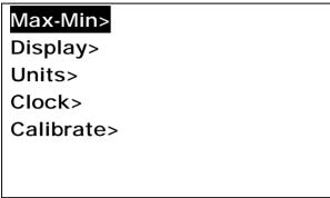
The first menu item "Max-Min" is highlighted, different menu items can be highlighted using the  $\acute{\mathbf{e}}$  and  $\acute{\mathbf{e}}$  buttons. The wanted action is done by highlighting the appropriate menu item and pressing the Set button. To abort without doing anything press the X button. In some cases a further sub-menu is displayed with more choices.
